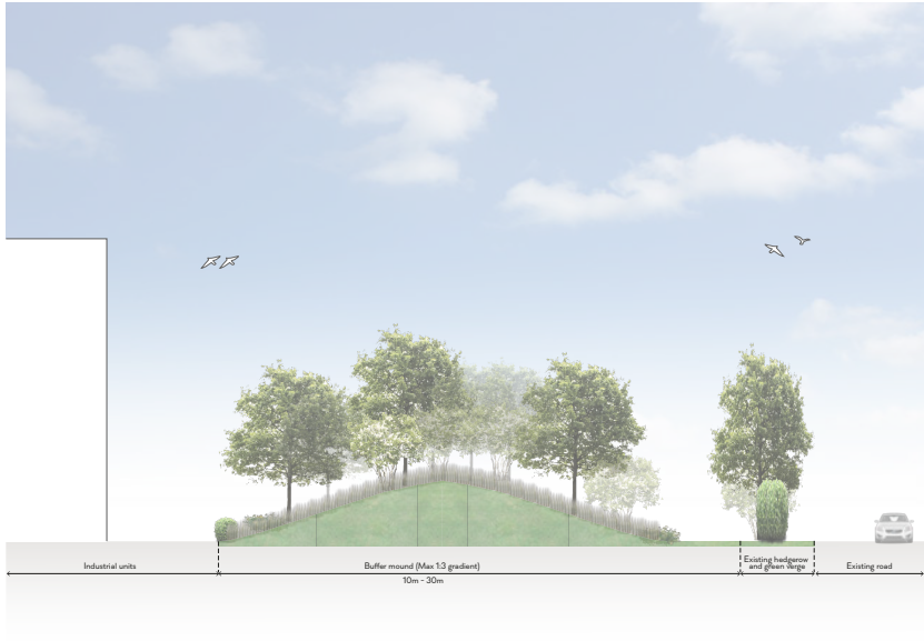
figure 36 | 1:500 | cross section b-b' landscaped bund to industrial context
